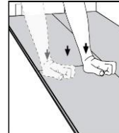
Figs 8c as it flattens itself to the floor press or gently tap the top of the short end of the installed panel until its flat. Finish installing this plank by tapping it with a tapping block on the long side to ensure secure installation.
