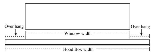
The left hand screw for the Hood Box should be places to the left of the top corner of the window at the attachment point of the over hang and 180mm higher (the height of the Hood Box). If installing on a brick wall NEVER put the screw into a mortar line. If the position you need to drill is over a mortar line move up to the bottom of the brick above that position.
