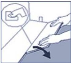
Fig 3. Angle the plank down. During the angle process make sure the planks are tight against each other. Afterwards press down or slightly tap down at the short end or long edge of the installed plank till its flat. No major force is or required, use a tapping block or piece of softwood to avoid edge damage.
