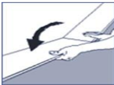
Fig 2. Second plank, first row angle long side & angle short end into place gently and tight to short end of first plank. Light hand pressure or a lengthways tap maybe required to secure tightly. Please make sure both long edges and short ends are tight with no visible gaps.
